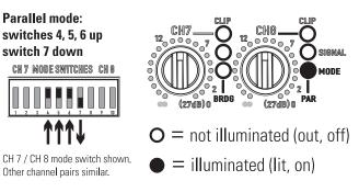
Mode switch settings and LED indication for parallel mode operation. PAR indicator should be illuminated and BRDG indicator should not be illuminated when in parallel mode.
